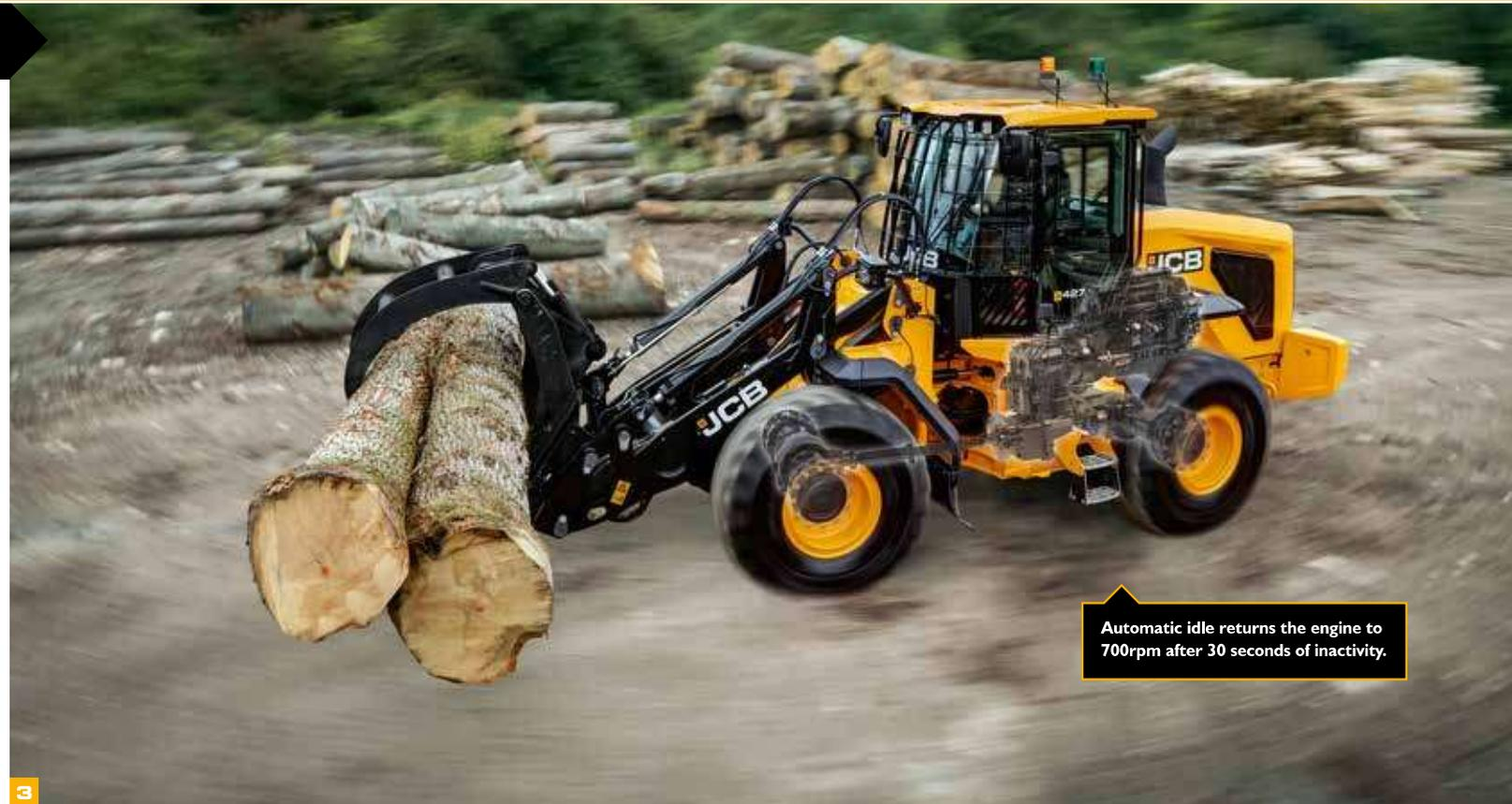
Automatic idle returns the engine to 700rpm after 30 seconds of inactivity.
